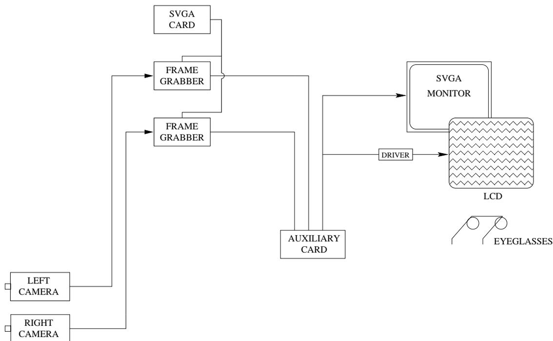
Fig. 2. Architecture of the stereo vision system.
